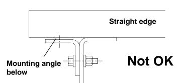
If the mounting angle is below the straight edge the slide plate will be bowed down. This bowing will bind the locking plungers. You must correct the mounting angle to ensure proper slider operation. Follow the procedures below.
