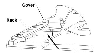
If the gage fits completely between the bracket and rack the bracket needs to be replaced.
