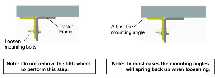
Step 1-7) After properly aligning the mounting angle tighten all mounting bolts to their proper torque.
