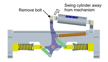
Step 3-3) Place a pipe over the pivot arm and open the release mechanism to break free the corrosion, dirt and debris.
