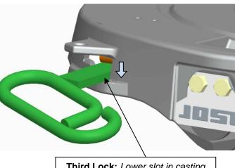
Third Lock: Lower slot in casting
