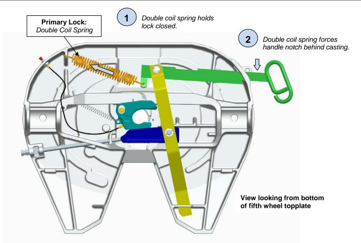
The release handle is secured when the secondary lock notch is behind casting skirt.
